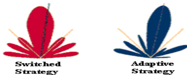
FIG 6: BEAM FORMING LOBES AND NULLS THAT SWITCHED BEAM (RED) AND ADAPTIVE ARRAY (BLUE) SYSTEMS MIGHT CHOOSE FOR IDENTICAL USER SIGNALS (GREEN LINE) AND CO-CHANNEL INTERFERERS (YELLOW LINES)
