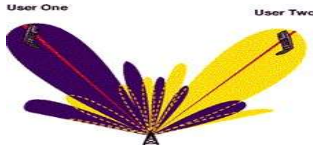
FIG 8: FULLY ADAPTIVE SPATIAL PROCESSING, SUPPORTING TWO USERS ON THE SAME CONVENTIONAL CHANNEL SIMULTANEOUSLY IN THE SAME CELL
