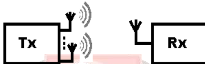
FIG 4: MISO - MULTIPLE INPUT SINGLE OUTPUTS
